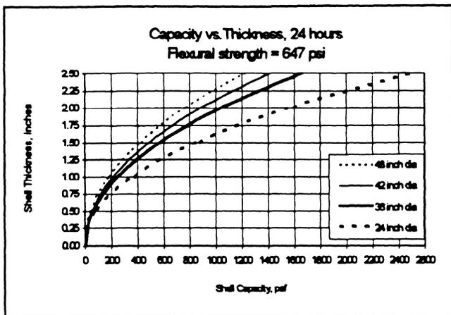
Figure 1. Moment load capacity of shells, 24 hour test
