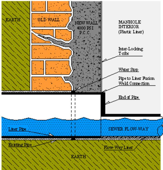
Typical cross section of **PERMAFORM**<sup>®</sup> manhole
