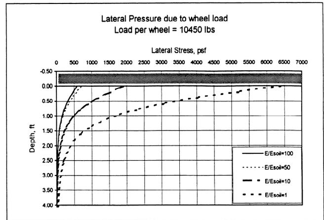
Figure 3. Lateral stresses due to wheel load
